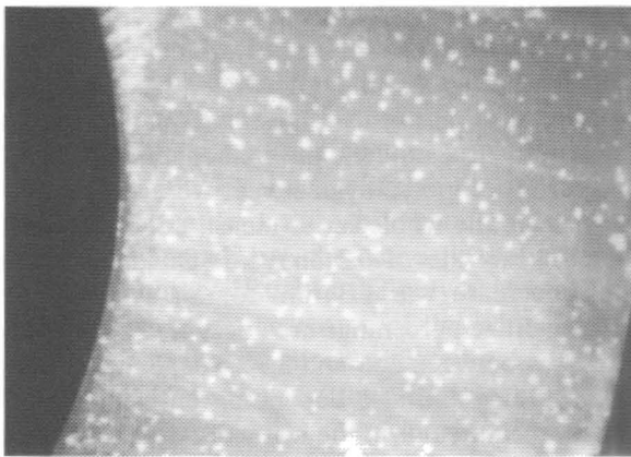
FIG. 2. This 200- \mu\text{m} slice of polyethylene shows the so-called fusion defects, also known as unconsolidated polyethylene particles
