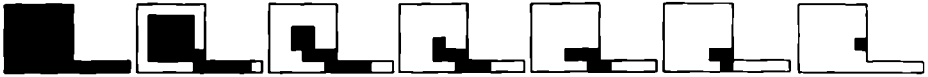
Fig. 2. Example, of voxel removal failure. If we use this technique on a vessel with an irregular section, the resulting centerline may be even composed by border voxels.
