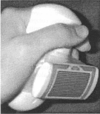
Fig. 1. Tactile Imaging scanhead used in this study. The working portion is an array of passive pressure sensors. When pressed gently and stroked over the tissue of interest it records higher pressures near stiffer regions, thus recording the palpable characteristics of the tissue
