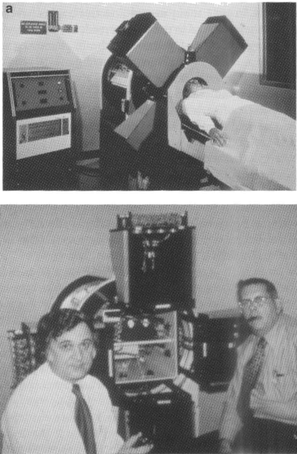
Fig. 6.2 (a) First tomographic radioisotope scanner, invented by David Kuhl at the University of Pennsylvania in the 1960s. The patient had a stroke, and the tracer was technetium-99m albumin. (b) Dr. David Kuhl and Dr. R. Q. Edwards. (c) Schematic drawing of the first tomographic scanner.
