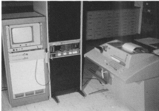
Fig. 7.6 The Image Display And Analysis System (IDA) built at Hopkins in 1968, one of the first minicomputers in nuclear medicine.
